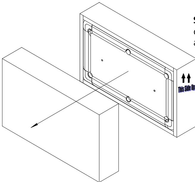
**Step #1** - Place the pool table box on its side, remove the banding and the top of the box.
