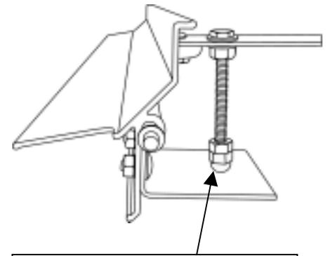
The acorn nut should be adjusted so it is just above the anti-cheat plate in the resting position. There needs to be enough space so that the F-bracket can move smoothly when the coin-mech is actuated.
