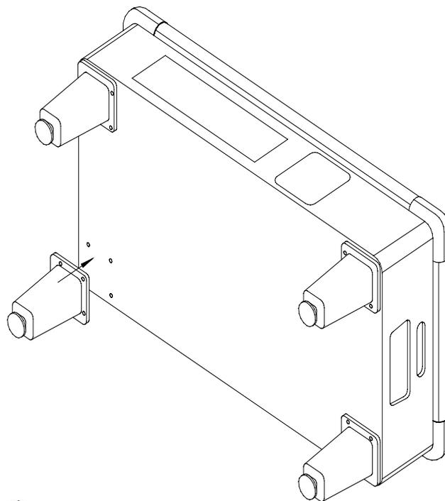
**Step #4** - Rough level the pool table by placing a level across, lengthwise, and diagonally into the four corners and raise or lower the appropriate leg leveler. Final level the pool table by dropping a ball onto the nose of the cushion rail and watch the drift of the ball as it comes to a stop. Raise or lower the appropriate leg leveler until the ball rolls true.
